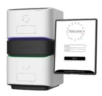
An example of POC/decentralized testing multidisciplinary multiplatform. Capabilities include cell counting, chemistry assays (electrolytes, small molecules, and proteins), and immunoassays (proteins). Promises rapid TAT and high performance at low cost.
